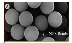
NPS® – An Ultra-Fast, high-resolution HPLC support tailored specifically for Peptides, Proteins & MS. The totally non-porous nature of NPS provides for fast mass transfer kinetics and high recovery of proteins at low surface carbon loads and organic MP modifiers. This allows for easy elution and recovery of highly hydrophobic proteins.
