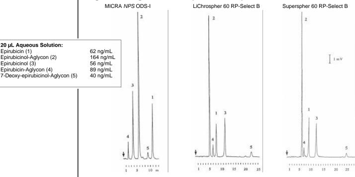
Operating Conditions - Fluorescence Detector; ex: 445nm, em: 560nm MICRA NPS ODS-I
