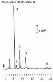
Coupled-column HPLC analysis consisting of a restricted access "Alkyl-Diol" silica (ADS) pre-column followed by the analytical column. Further information regarding this analysis may be obtained by contacting Eprogen, Inc.
